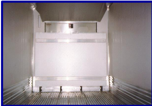
Clean trailer w/ attached air chute
